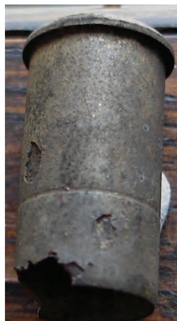
Figure 6.156. Partial corrosion fingerprint on spent brass shell casing, visualized following the application of a high potential and conducting powder.
