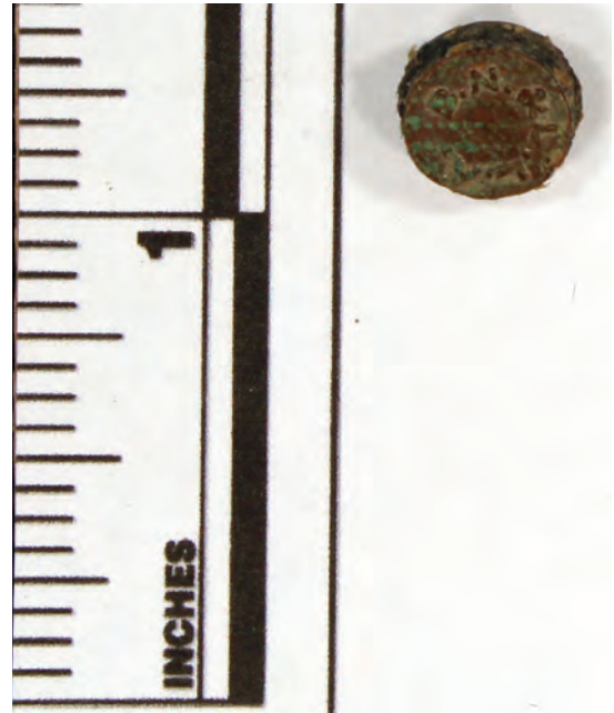
Figure 6.111. Rivet from NH89A with "B.N. & L.L.A." trademark.
