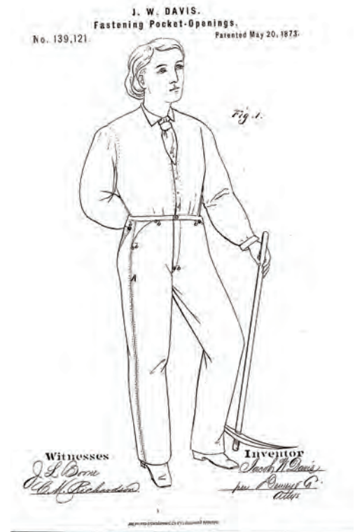
Figure 6.110. Jacob Davis’s “Improvement in fastening pocket-openings” patent illustration.
