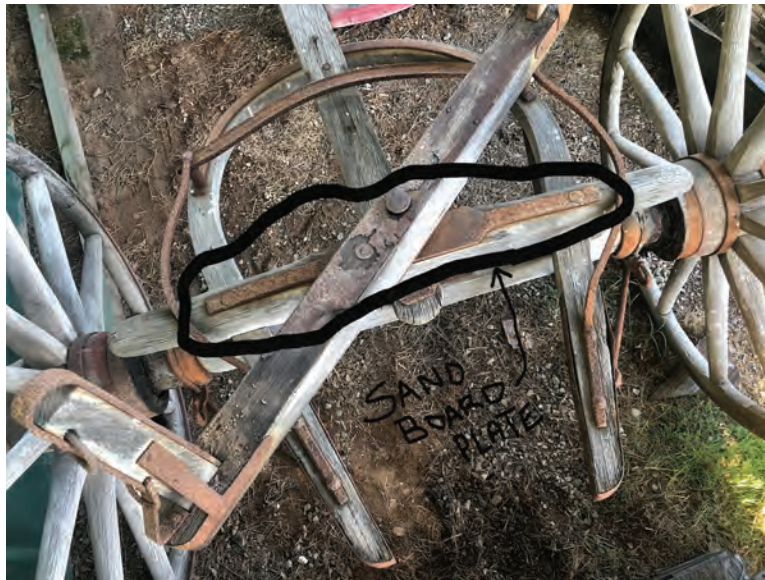
Figure 8.66. The sand board plate sits above the sand board and is circled and labeled in black in this plan-view photograph of a currently assembled historic wagon. (Courtesy David Sneed)
