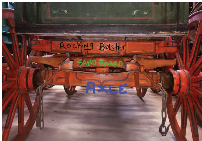
Figure 8.67. The sand board plate is between the rocking bolster and the sand board and axle in this labeled profile-view photograph of a currently assembled historic wagon. (Courtesy David Sneed)
