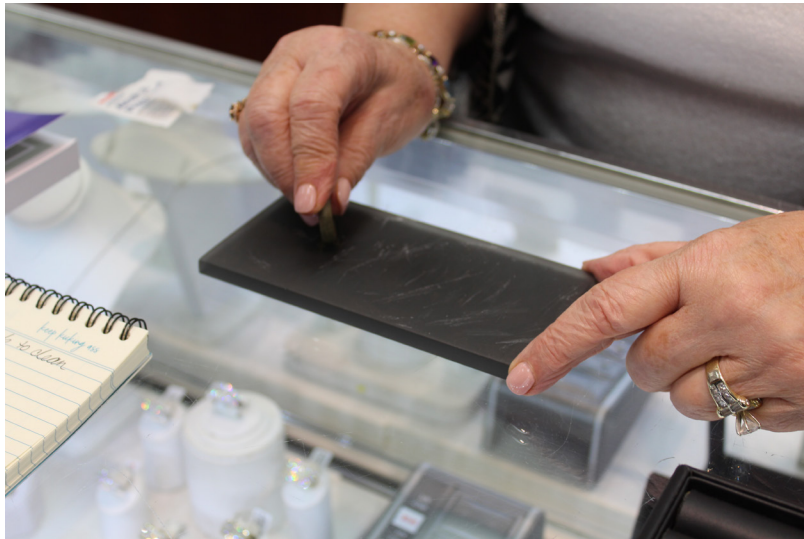
Figure 9.75. Kathleen White rubbing ring on testing plate (Courtesy Nathan Harrison Historical Archaeology Project).
